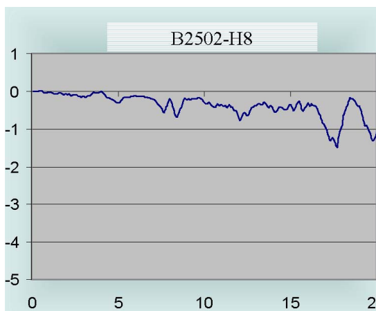
Figure 1: Insertion Loss, S21, B2502-H8
