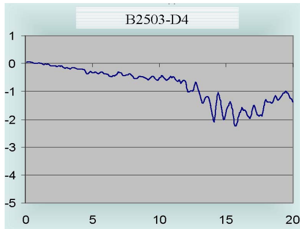
Figure 3: Insertion Loss B2503-D4
