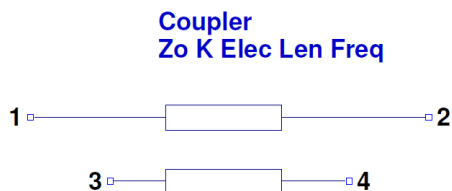
Figure 8: Transmission Line Equivalent for Crosstalk
