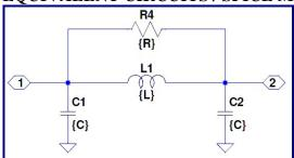
Figure 5: Pi Equivalent, Valid to 10GHz
