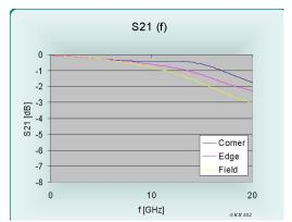
Figure 6: Insertion Loss, S21, B2501-L3
