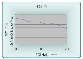
Figure 5: Insertion Loss, S21, B2501-A1
