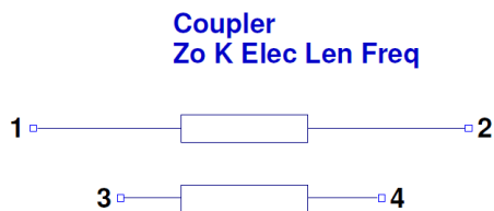
Figure 8: Transmission Line Equivalent for Crosstalk
